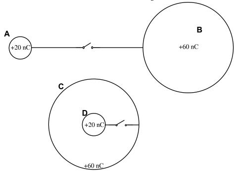
Rank the electric charge on the shells A-D after the switches are closed.
