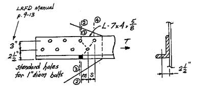
Failure through the open hole is computed using section 2-2 with 6/8 of the load acting (the open hole is not involved in load transmission). If m is small, failure may be through three holes with 100% of load.
