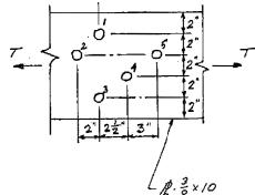
Section 1-2-3 with two stagger paths:  $A_n = A_g$  -3holes + 2staggers
