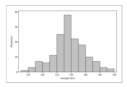
The histogram of ultimate strengths is symmetric and unimodal, with the point of symmetry at approximately 135 ksi. There is a moderate amount of variation, and there are no gaps or outliers in the distribution.
