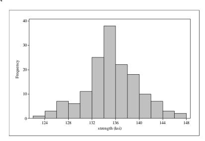
The histogram of ultimate strengths is symmetric and unimodal, with the point of symmetry at approximately 135 ksi. There is a moderate amount of variation, and there are no gaps or outliers in the distribution.
