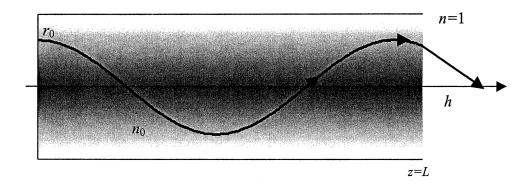
For an incident ray parallel to the axis with an initial position of  $r_0$  at z = 0, the ray path is given by
