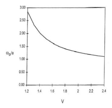
The magnitude of  $\omega$  /a increases gradually and then more rapidly as the normalized frequency, V, is reduced below 2.4. Hence the light initially (at V = 2.4) occupies the whole of the fiber core and as V is reduced the spot size expands further into the cladding region such that below a normalized frequency of 1.4 it occupies an area which is greater than four times the core region.
