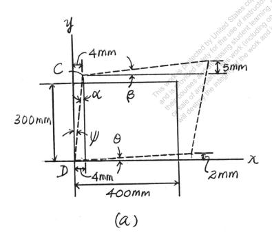
Ans:  $(\gamma_{xy})_C = 25.5(10^{-3}) \text{ rad}$  $(\gamma_{xy})_D = 18.1(10^{-3}) \text{ rad}$  \*2-12.
