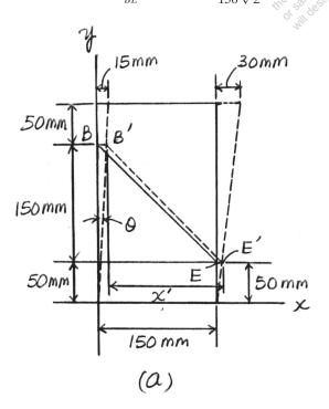
**Ans:**  $(\epsilon_x)_A = 0$   $(\epsilon_y)_A = 1.80(10^{-3}) \text{ mm/mm}$   $(\gamma_{xy})_A = 0.0599 \text{ rad}$   $\epsilon_{BE} = -0.0198 \text{ mm/mm}$
