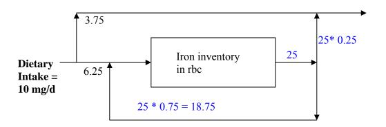
Equation 2.5 works where  $M_i = 10$ ,  $M_d = 25$ , and  $\varepsilon = 0.75$ . Or the easier way of using inspection can be pursued if one understands how the bodily processes map onto the flow sheet. Numbers are shown on Figure when inspection is used.
