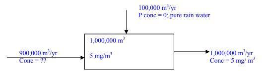
Mass flow P in = mass flow P out at steady state, and volumetric flow rate of water into the lake will maintain constant lake volume
