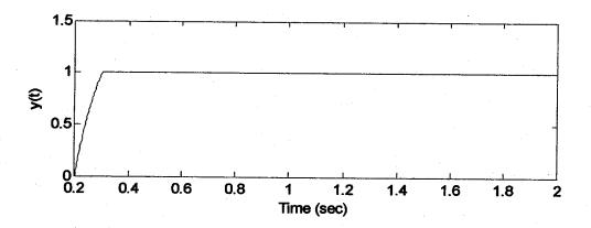
From the above plots, we see that the eye does lock onto the target for all three values of b. However, when b = 1, there is overshoot, and when b = 0.2, the response is somewhat slow in reaching the steady-state value. The best result is obtained when b = 0.582, which is the value of b computed analytically in Part (b) of Problem 2.35.
