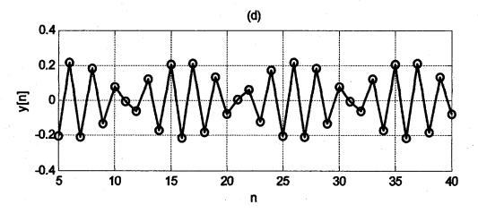
(e) The signal in Part (d) has a much higher frequency than that of the sinusoidal signal in Part (c). Since the 5-point EWMA flter is a "lowpass filter," it attenuates the high- frequency signal in Part (d), while it passes the low-frequency signal in Part (c) with very little attenuation.
