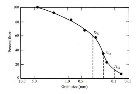
b. From the graph,  $D_{60} = 0.3 \text{ mm}$ ;  $D_{30} = 0.17 \text{ mm}$ ;  $D_{10} = 0.11 \text{ mm}$
