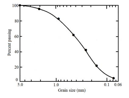
b. From the graph,  $D_{60} = 0.4 \text{ mm}$ ;  $D_{30} = 0.22 \text{ mm}$ ;  $D_{10} = 0.12 \text{ mm}$
