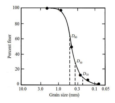
b. From the graph,  $D_{60} = 0.48 \text{ mm}$ ,  $D_{30} = 0.33 \text{ mm}$ ,  $D_{10} = 0.23 \text{ mm}$
