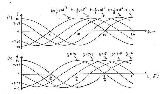
f(z, t) represents a traveling wave progressing with time in the negative z-direction.
