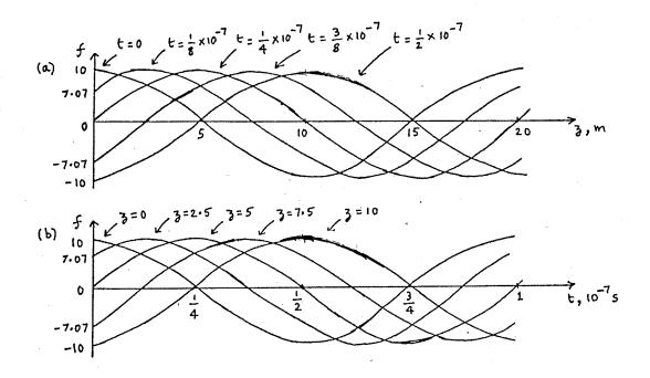
f(z, t) represents a traveling wave progressing with time in the positive z-direction.
