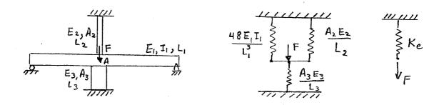
From Table 4.1, the Ke for the beam is:
