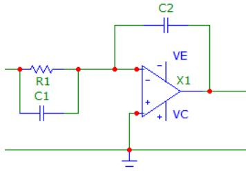
$$\frac{-Z_f}{Z_i} = -\left( \frac{C_1}{C_2} + \frac{1}{R_1 C_2 s} \right) = -\left( 10 + \frac{0.1}{s} \right) \Rightarrow \frac{C_1}{C_2} = 10, \quad R_1 C_2 = 10 \text{ s} \quad \text{Let } R_1 = 1M\Omega, \text{ then } C_2 = 10\mu F, \text{ and } C_1 = 100\mu F.$$
