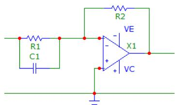
$$\frac{-Z_f}{Z_i} = \frac{-R_2(1 + R_1 C_1 s)}{R_1} = -\left(\frac{R_2}{R_1} + R_2 C_1 s\right) = -(10s + 1) \Rightarrow R_f C_1 = 10, \quad \text{let } R_2 = R_1 = 100K, C_1 = 100\mu F.$$
