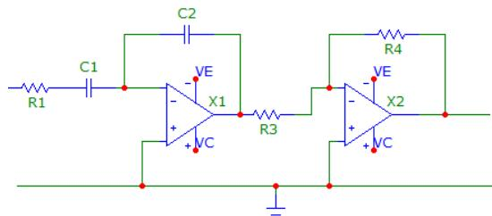
Let  $R_3 = R_4 = 100K$ . Gain = -1 for second stage. For first stage,
