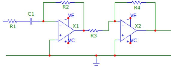
Let  $R_3 = R_4 = 100K$ . Gain = -1 for second stage. For first stage,
