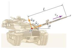
which shows that the contribution to v due to the angular velocity of the barrel is negligible compared to  $v_s$ .
