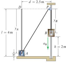
where we have used the fact that  $\ddot{y}_B = a_0 = 5.7 \text{ m/s}^2$  and h = 2 m. Then, using Eq. (5) and the last of Eqs. (7), and recalling that d = 2.5 m, we can evaluate Eq. (6) to obtain for  $t = t_f$  to obtain
