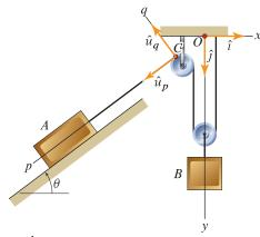
Determine the speed of block B if block A is sliding down the incline with a speed  $v_A = 1.5$  m/s while the cord is retracted by a winch at a constant rate  $v_0 = 2.5 \,\mathrm{m/s}.$
