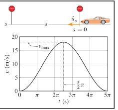
The following four problems refer to a car traveling between two stop signs, in which the car's velocity is assumed to be given by  $\hat{u}_s$ 0 S  $v(t) = [9 - 9\cos(2t/5)] \text{ m/s for } 0 \le t \le 5\pi \text{ s.}$ s = 0Determine the time at which the brakes are applied and the car 20 starts to slow down. v<sub>max</sub> 15 (s/m) n 5  $\frac{5}{2}\pi$ 00  $2\pi$ π  $3\pi$  $4\pi$  $5\pi$ t (s)
