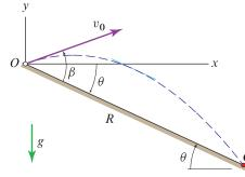
Parameters = {g  $\rightarrow$  9.81,  $\theta \rightarrow$  25. Degree, R  $\rightarrow$  7.}; Plot  $\left[\sqrt{\frac{gR}{2}} \frac{\cos[\theta]}{\sqrt{\sin[\beta]\cos[\beta - \theta]}}$  /. Parameters, { $\beta$ , 0, 2}, Frame  $\rightarrow$  True,
