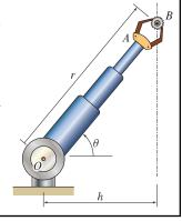
As a part of an assembly process, the end effector at A on the robotic arm needs to move the gear at B along the vertical line shown with some known velocity  $v_0$  and acceleration  $a_0$ . Arm OA can vary its length by telescoping via internal actuators, and a motor at O allows it to pivot in the vertical plane.
