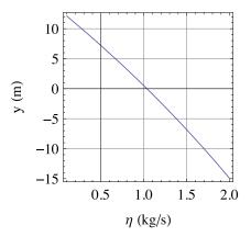
From the plot above, we see that y = 0 for  $x = (x_I)_{air}$  when  $\eta$  is a bit greater than 1 kg/s. Hence, we will use the value  $\eta = 1$  kg/s as the guess for a root finding algorithm in order to find a more accurate value of the value of  $\eta$ . When using Mathematica, this can be done with the following code
