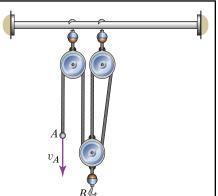
In maritime speak, the system in the figure is often called a *whip-upon-whip purchase* and is used for controlling certain types of sails on small cutters (by attaching point *B* to the sail to be unfurled). If the end of the rope at *A* is pulled with a speed of 4 m/s, determine the velocity of *B*. Neglect the fact that the segment of the rope between *C* and *D* is not vertically aligned, and assume that the slope of segment *AC* is constant.
