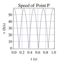
**Velocity Components** The components of the velocity of *P* can be plotted for  $0 \le t \le 1$  s using the expressions in Eq. (2) with  $v_0 = 20$  mph = 29.33 ft/s and R = 1.15 ft. The plot shown below was generated using *Mathematica* with the following code:
