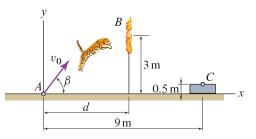
where, again recalling that  $(x_B, y_B) = (5.5, 3)$  m and  $(x_C, y_C) = (9, 0.5)$  m, we have evaluated  $v_0$  by first evaluating  $C_2$  in the last of Eqs. (3) and then the angle  $\beta$  in the last of Eqs. (4). Now that  $v_0$  and  $\beta$  are known, observing that  $\vec{v}_{initial} = v_0 \cos \beta \hat{i} + v_0 \sin \beta \hat{j}$ , we can evaluate  $\vec{v}_{initial}$  to obtain
