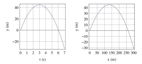
From the above two plots, we see that  $t_I$  is close to 6 s and  $x_I$  is close to 250 m. Hence, we will use the values just listed as guesses in an appropriate root finding numerical method to find more accurate values to the quantities  $t_I$  and  $x_I$ . For example, this can be done using *Mathematica* with the following code:
