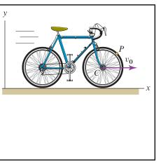
A bicycle is moving to the right at a speed  $v_0 = 20$  mph on a y horizontal and straight road. The radius of the bicycle's wheels is R = 1.15 ft. Let *P* be a point on the periphery of the front wheel. One can show that the *x* and *y* coordinates of *P* are described by the following functions of time:
