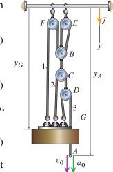
In the pulley system shown, the segment AD and the motion of A are not impeded by the load G. Assume all ropes are vertically aligned.
