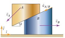
At the instant shown,  $\vec{v}_B = 5 \hat{i}$  m/s. If  $\theta = 25^\circ$ , determine the speed of A relative to B in order for A to travel only in the vertical direction while sliding over B.
