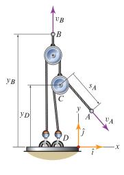
The pulley system shown is used to store a bicycle in a garage. If the bicycle is hoisted by a winch that winds the rope at a rate  $v_0 = 5$  in./s, determine the vertical speed of the bicycle.
