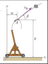
A trebuchet releases a rock with mass m = 50 kg at point O. The initial velocity of the projectile is  $\vec{v}_0 = (45 \hat{i} + 30 \hat{j}) \text{ m/s}$ . Neglecting aerodynamic effects, determine where the rock will land and its time of flight.
