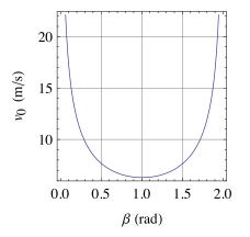
We can find the optimal value of  $\beta$  to reach a distance of R = 7 m by differentiating  $v_0$  with respect to  $\beta$  and setting it equal to zero. Recalling that  $\theta = 25^\circ$ , this gives
