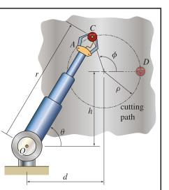
In the cutting of sheet metal, the robotic arm OA needs to move the cutting tool at C counterclockwise at a constant speed  $v_0$ along a circular path of radius  $\rho$ . The center of the circle is located in the position shown relative to the base of the robotic arm at O.
