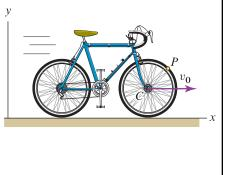
$x(t) = v_0 t + R \sin(v_0 t/R)$  and  $y(t) = R[1 + \cos(v_0 t/R)].$
