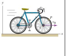
$x(t) = v_0 t + R \sin(v_0 t/R)$  and  $y(t) = R [1 + \cos(v_0 t/R)].$
