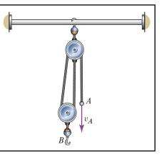
The gun tackle shown is operated with the help of a horse. If the horse moves to the right at a constant speed of 7 ft/s, determine the velocity and acceleration of B when the horizontal distance from B to A is 15 ft. Except for the part of the rope between C and A, neglect the fact that some portions are not vertically aligned. Also neglect the change in the amount of rope wrapped around pulley C as the horse moves to the right.
