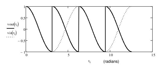
The output fundamental radian frequency is  $2\omega$ . Let's do the Fourier component for the fundamental in some detail.
