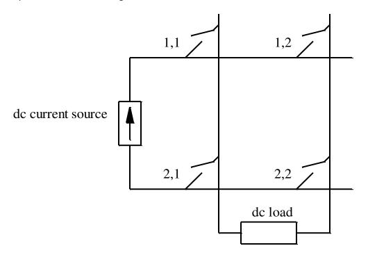
In this case only the KCL constraints are sought and the load requirements are not specified. KCL requires a current path. This in turn means that at least one switch must be on in each row. The allowed combinations based on KCL are:
