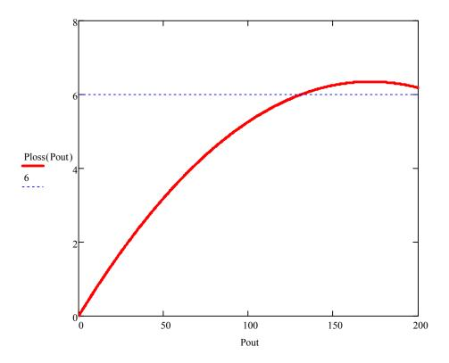
So there is a maximum output power between 100 W and 150 W that is the requested upper limit. The actual value is obtained by solving (3) for a value of 6 W, giving
