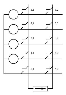
(b) KVL requires that unlike voltages do not become connected. This means that at most one switch in each column is allowed on at any time. In terms of switching functions,
