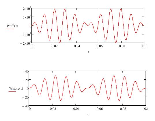
The peak storage need based on a 50 A current is about 29 J, as per the above computation.
