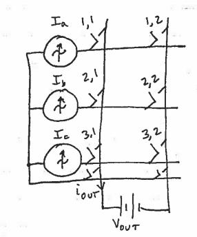
Notice that one and only one switch in each <u>row</u> should be on at a time.  $g_{11} + g_{12} = g_{21} + g_{22} = g_{31} + g_{32} = 1 = g_{41} + g_{42}$
