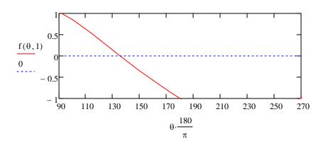
The diode turns off at about 135 degrees for this specific case.
