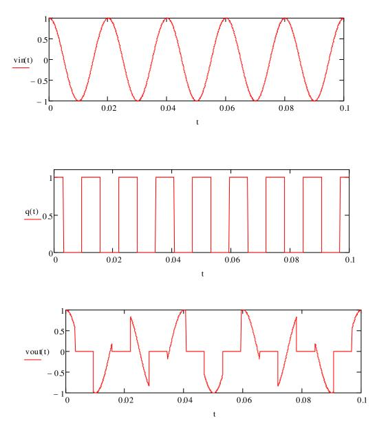
This waveform repeats every 0.1 s, and therefore has a frequency of 10 Hz. (Notice that 10 is the greatest common divisor of 50 and 80.)
