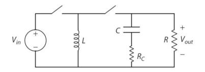
In this problem, the output voltage is not constant. As in prior energy methods, we expect the inductor current and capacitor voltage not to change much. Define a voltage vout1 with the left switch on and vout2 with the right switch on. Also define a capacitor current, directed down, with a value ic1 when the left switch is on and ic2 when the right switch is on. Define inductor current IL directed down and voltage Vc with positive at the top. The energy balance on the inductor is as follows:
