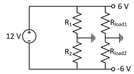
The total load can be up to 2 W in any fraction. For example, if the +6 V supply provides 2 W and the -6V provides 0 W, then  $R_{load1}$  will be 18  $\Omega$  and  $R_{load2}$  will be infinite (open). If each supplies 1 W, the resistors are 36  $\Omega$ , and so on.
