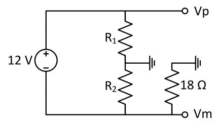
Case 2:  $R_{load1} = 18 \Omega$ ,  $R_{load2} = infinite$
