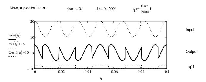
This shows the output (solid), the input (dotted, with an offset for clarity), and q11. By inspection, the output waveform repeats every 0.05 s, giving a fundamental frequency of 20 Hz.
