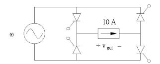
The figure shows a bridge with an arbitrary current source load, modified to use SCRs in place of diodes. The SCR allows us to delay the turn-on. An SCR is off unless a gate signal is applied, and then acts like a diode. For the trial method, this means we can treat the device as fully blocking when no gate signal is present, and as a diode once a gate signal (even a brief one) is applied.
