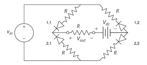
This is a trial method problem. Choose a configuration and test for consistency. The diodes have had numerical labels added above for convenience.
