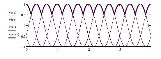
What is the average value? The waveform is periodic with a period 1/3 that of each input. Define a change of variables  $\theta = \omega$  t, then the period is  $2\pi/3$  radians and the average becomes
