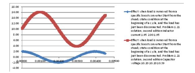
Now one can argue that this analysis was not very instructive. A more typical situation comes into play in most real implementations of boost converters. In these circuits, energy flows only in one direction, from input to output. The inductor current will not become negative and energy will not be exchanged between the inductor and capacitor. What happens in this case when the load is disconnected?
