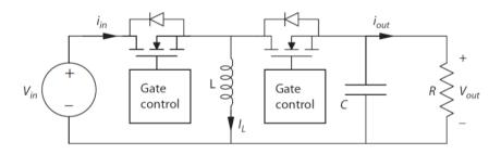
Notice that if initially iL = vC = 0, when the left switch is turned on, voltage Vin is imposed on the inductor and the current will rise. After that, the right switch turns on by vC = 0 and so the inductor current will stay constant in principle, but in fact current will be pulled out of the capacitor, drawing its voltage slightly negative.
