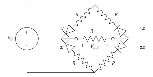
This is a trial method problem. Choose a configuration and test for consistency. The diodes have had numerical labels added above for convenience.
