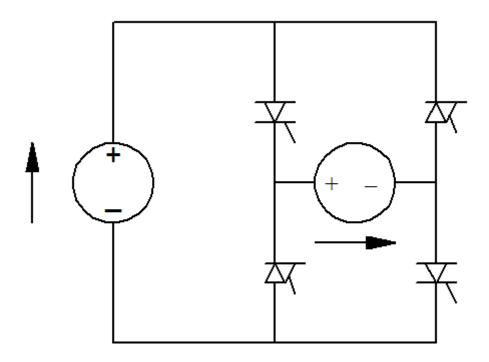
As shown, all four devices require gates. This switch matrix will be able to implement any unipolar dc-dc converter, whether the input is a voltage source (with output current source) or the input is a current source (output voltage source).
