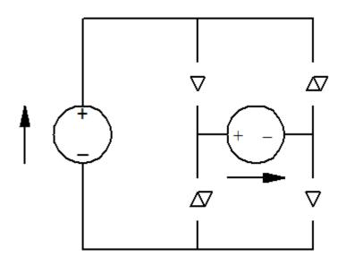
What about voltage? Switch 1,1 could be asked to block the input voltage when off. This would require a blocking "line" at the top. However, with switch 1,2 on, switch 1,1 could be required to block the output voltage, which would require reverse blocking. The same arguments apply to switch 2,2. Therefore both of these must block bidirectional voltage.
