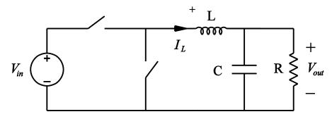
To determine the ratio for 50% on time for the left switch, perform an energy balance on the inductor. The voltage on the inductor is  $V_{in}$  - $V_{out}$  with the left switch on and - $V_{out}$  with the right switch on. Energy balance is required. Over a full cycle, the net energy into the inductor must be zero.
