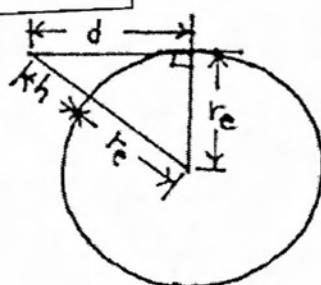
$$\begin{aligned} (h+r_e)^2 &= d^2 + r_e^2 \\ \Rightarrow h^2 + 2hr_e &= d^2 \text{ where } h \ll r_e \\ \Rightarrow d^2 &\approx 2hr_e \text{ and } r_e = \frac{4}{3}(3960 \text{ miles}) = 5280 \text{ miles} \\ \text{Let } h &= \text{antenna height in feet, and } d \text{ in miles.} \\ \Rightarrow d^2 (\text{miles})^2 &\approx 2h \left(\frac{1 \text{ mile}}{5280 \text{ feet}}\right) (5280 \text{ miles}) \\ \Rightarrow d^2 &= 2h \text{ or } \underline{\underline{d = \sqrt{2h}}} \end{aligned}$$
