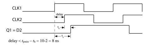
(b)  $t_{clk} \ge t_{pmin} + t_{su} = 15 + 4 = 19$  ns. (worst case occurs when delay = 0)
