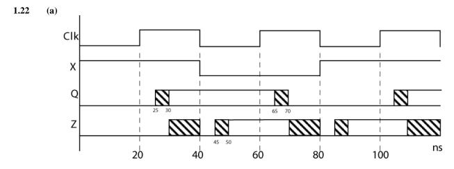
(b) Setup time = 20 ns -10 ns = 10 ns (due to change in X) Hold time =  $t_{pmin} + t_{pla} = 5$  ns+ 5 ns= 10 ns (due to change in Q)
