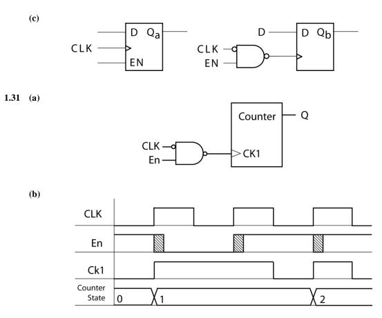
The clock input to the NAND gate in (a) is inverted. After the rising edge of the clock, this input to the NAND gate is a '0', so CK1 will remain a constant '1', regardless of any changes that may occur in the EN input of the gate due to transients.
