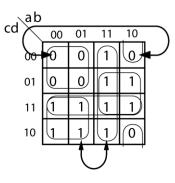
$$F = ((ab)'.(a+c)'+(a'+d)')' = ab + ((a+c)'+(a'+d)')' = ab + (a + c)(a' + d) = ab + aa' + ad + a'c + cd;$$
