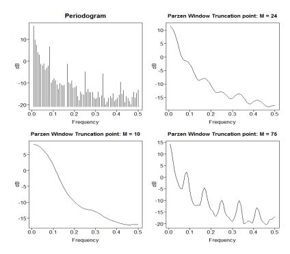
All spectral estimator have a peak at zero, and all except M=10 show the peaks at the harmonic of the fundamental frequency 1/12. The spectral estimator that is closest to the AR spectral estimator in Figure 1.25 is the Parzen spectral estimator with M=75. The Parzen spectral estimator with M=10 is clearly too smooth.
