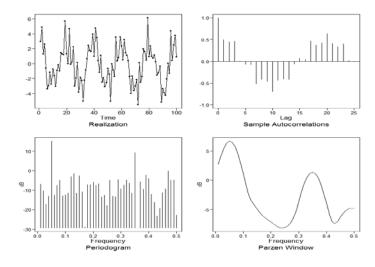
The realizations shows a dominant frequency with period about 20 along with higher-frequency behavior. The autocorrelations show the periodic behavior of associated with the period 20 (f=0.05) with some indication of a higher frequency component. These two plots provide very little evidence regarding the nature of the higher frequency behavior. The two spectral plots clearly suggest frequency behavior at both f=0.05 and f=0.35.
