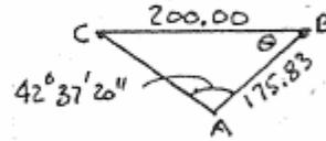
$$\frac{\sin C}{175.83} = \frac{\sin 42^\circ 37' 20''}{200} \rightarrow C = 36.5359^\circ \\ \theta = 180^\circ - 42^\circ 37' 20'' - C = 100.8419^\circ$$
