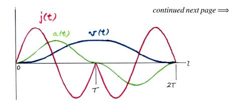
(b) The speed v(t) is the area under the curve of a(t). As the sketch indicates, v(t) increases with time up to t = T, and then decreases. The maximum speed  $v_{max}$  therefore occurs at t = T, so that  $v_{max} = v(T)$ .
