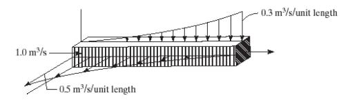
Using the development presented in the solution for Prob. 2.14, the volume flow rate at any station along the duct is:
