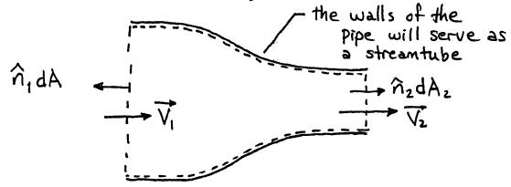
The vectors representing the areas (ridA) are directed outward from the control volume, as shown in the sketch. The velocities represent an assumed flow from left to right. Using the vector dot products and noting that the flow properties do not vary across the cross-section, we obtain:
